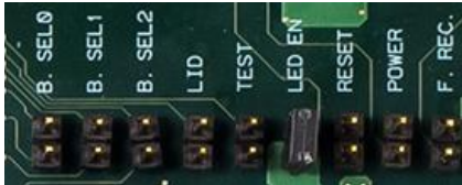
Figure 50: Jumpers for Boot Select
