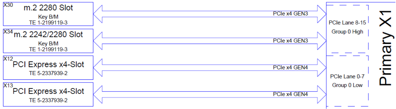
Figure 11: PCIe x4 Slots
